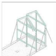
10. Hold the frame in place with supporting studs
